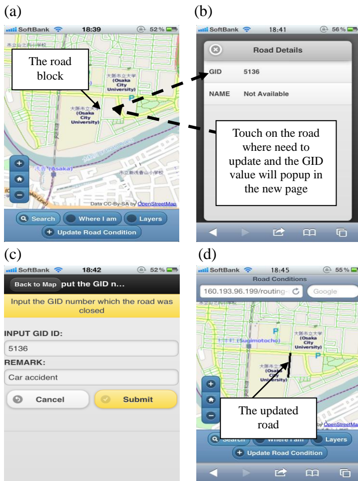
Figure 4. Show the updating road interface (accident point) to hospital D is computed. Figure 5(b) presents the new routing result after the road condition was updated.
